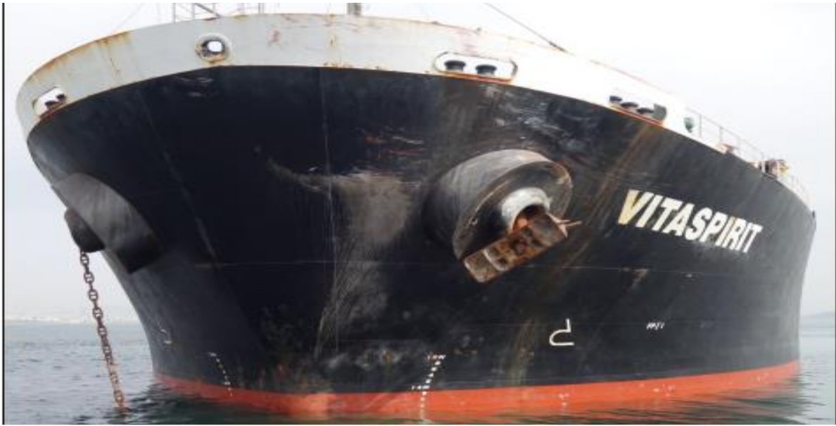
Figure 10: Superficial bow damage
