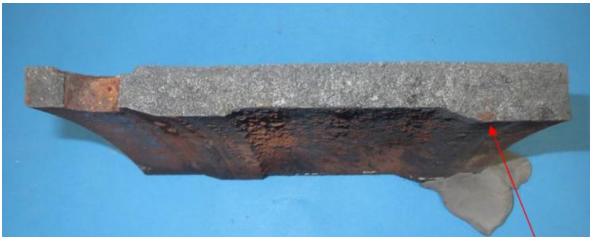
Figure 13a: Fracture surface after flash, inhibited acid cleaning (Clarke Solution). Rust was removed save for a small area close to the lower seal end.
