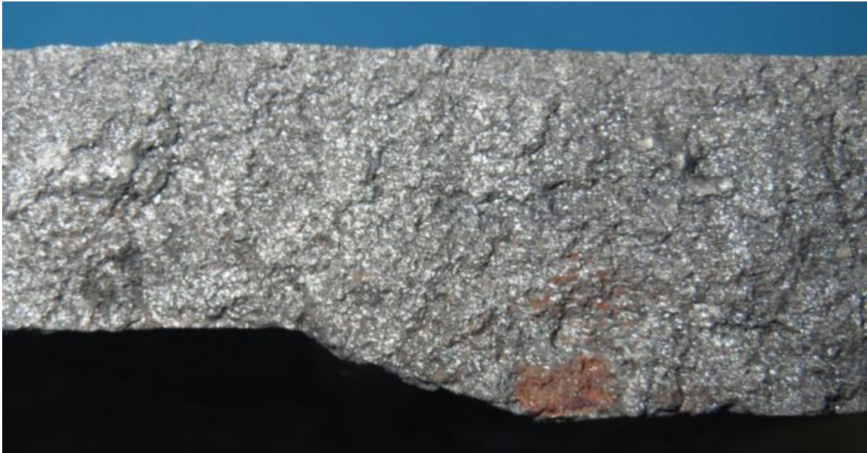
Figure 13b: Closer view showing the fracture surface after flash, inhibited acid cleaning and the small area of rust-affected fracture surface
