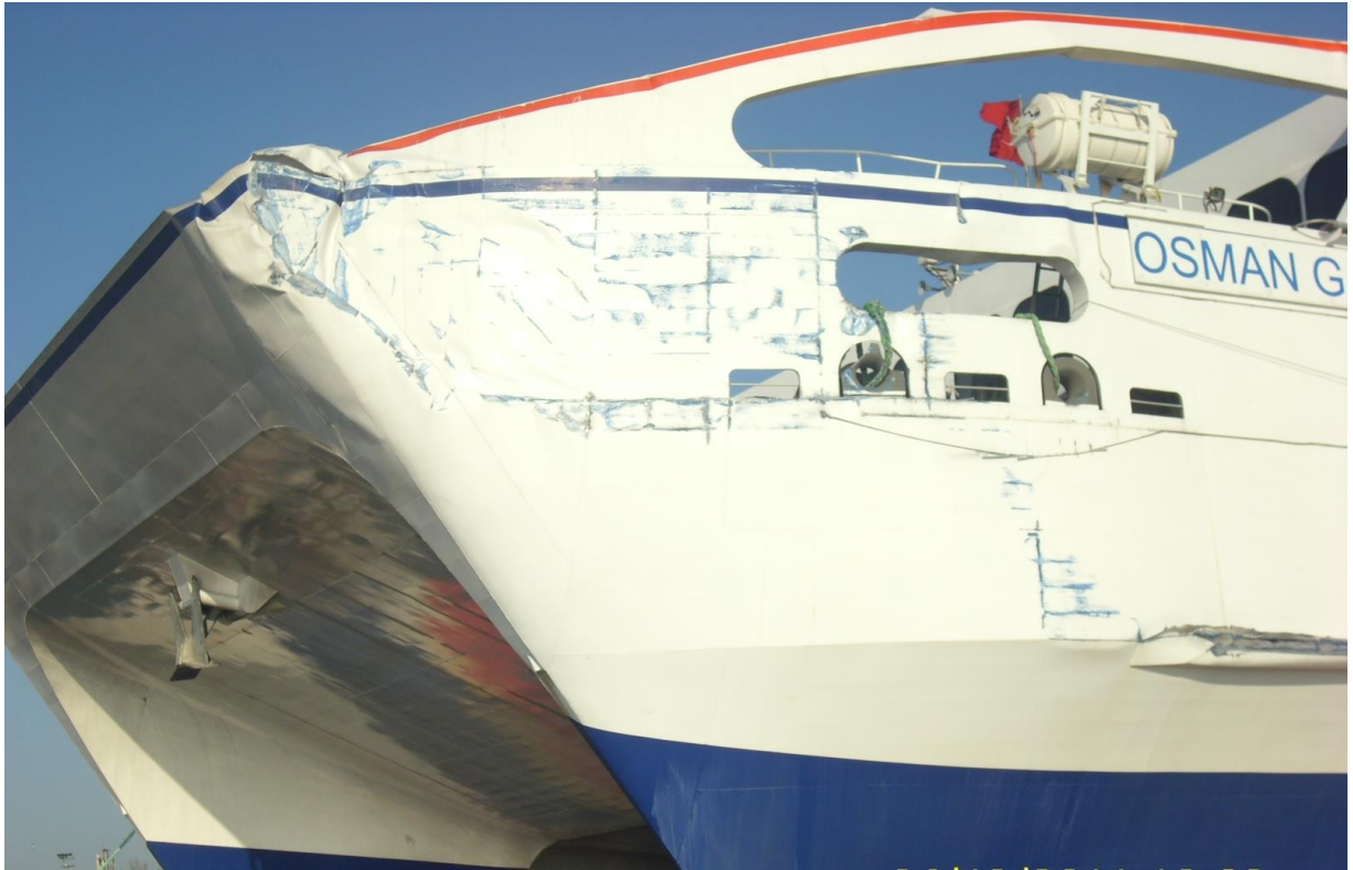
Figure 6: Damage to port bow of OSMAN GAZI-1
