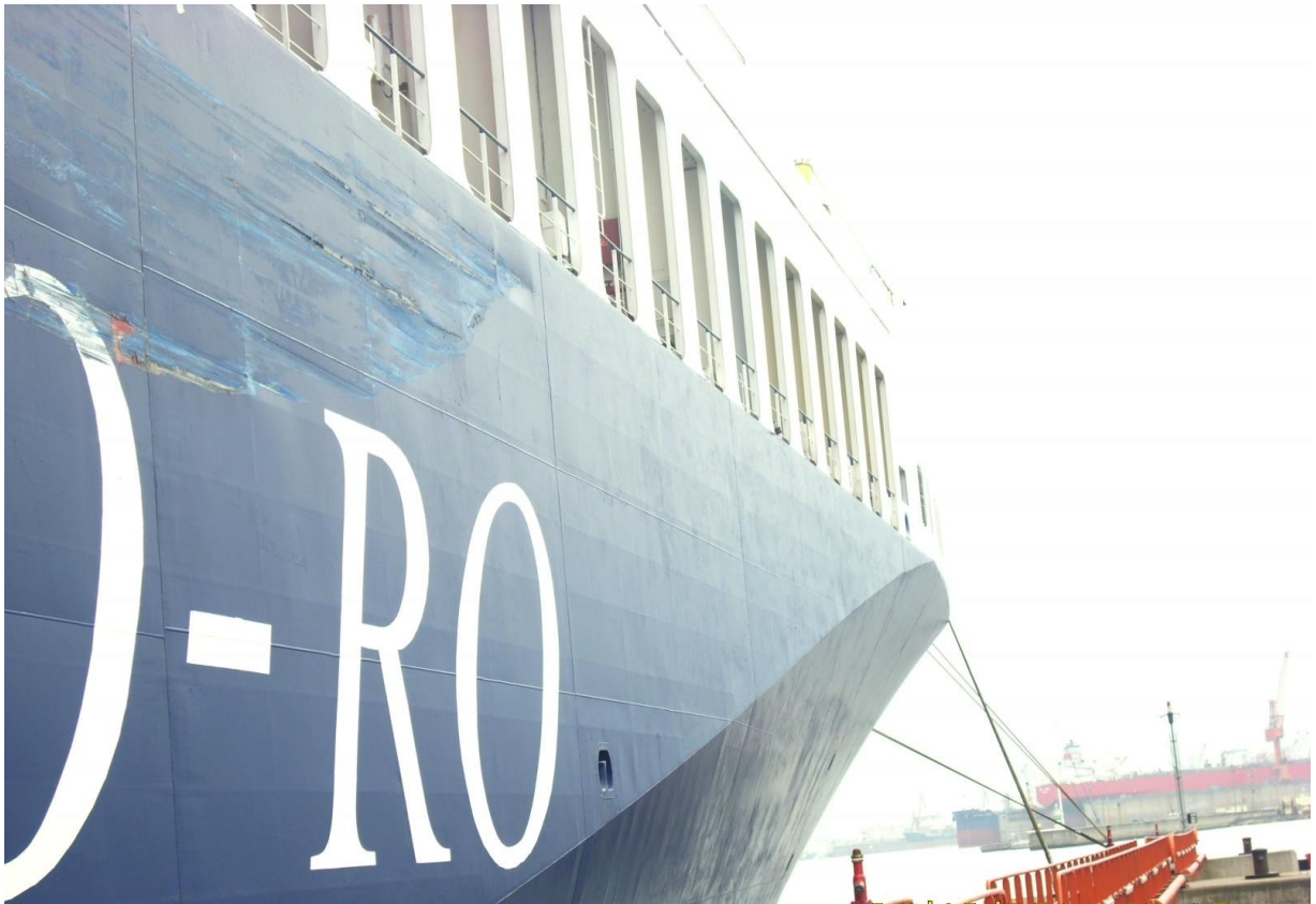
Figure 4: Damage to starboard beam of UND EGE
