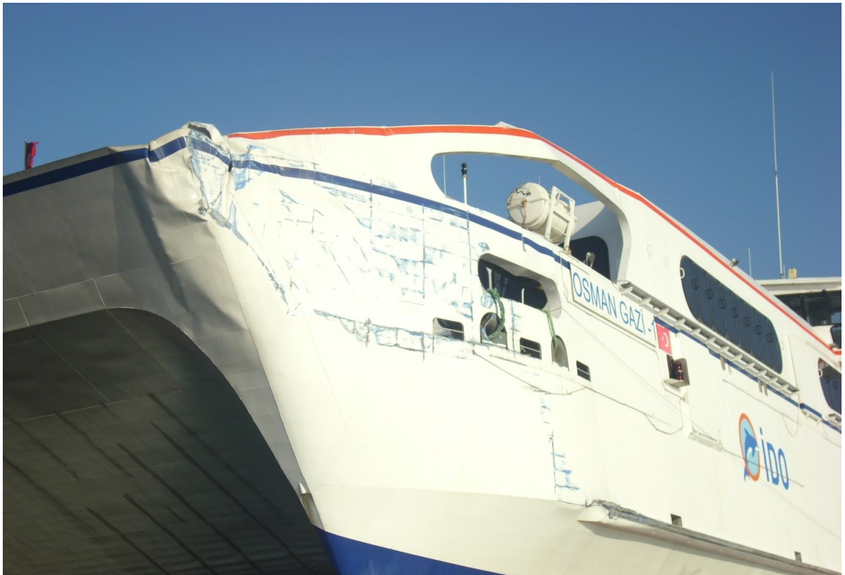
Figure 7: Damage to starboard bow of OSMAN GAZI-1
