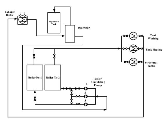
*Line Diagram 1 Boiler Line Diagram of the M/T TORC (Concept)*
