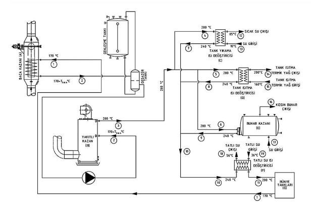
Line Diagram 2 Similar Thermal Oil Boiler Line Diagram
