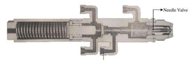
Image 10 Cross Section of Nozzle Unit
