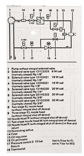
Line Diagram 3 Line Diagram of the Burner RMS9
