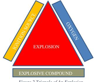
Figure 2 Triangle of An Explosion
