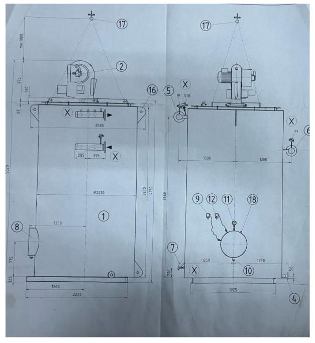
Figure 4 Connections and Components of Boiler Body
