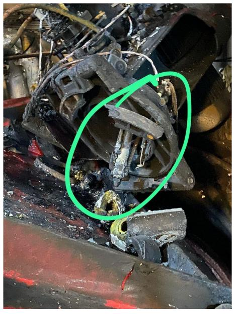
Image 9 Nozzle and Electrodes as a Result of Explosion
