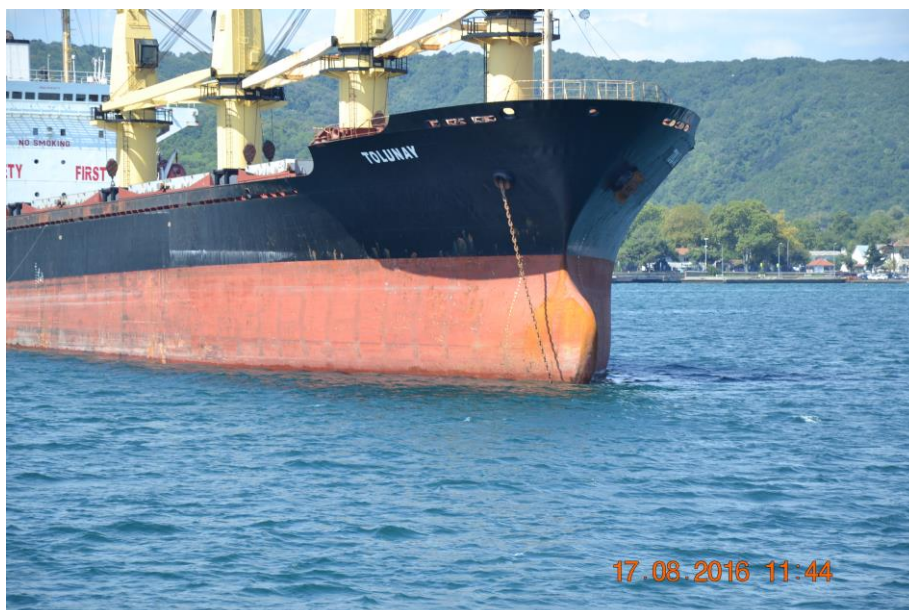
Picture 15: The damage at the Bulbous Bow of MV TOLUNAY after the collision
