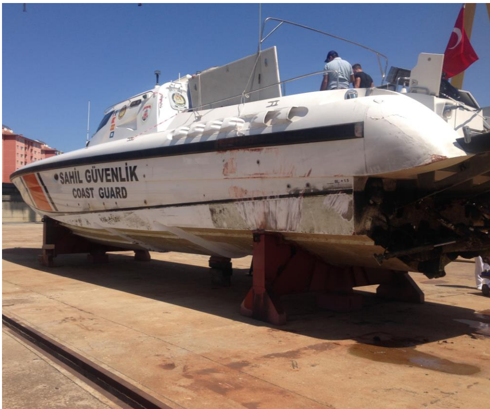
Picture 13: The damage at the Port Quarter of TCSG 25 Boat
