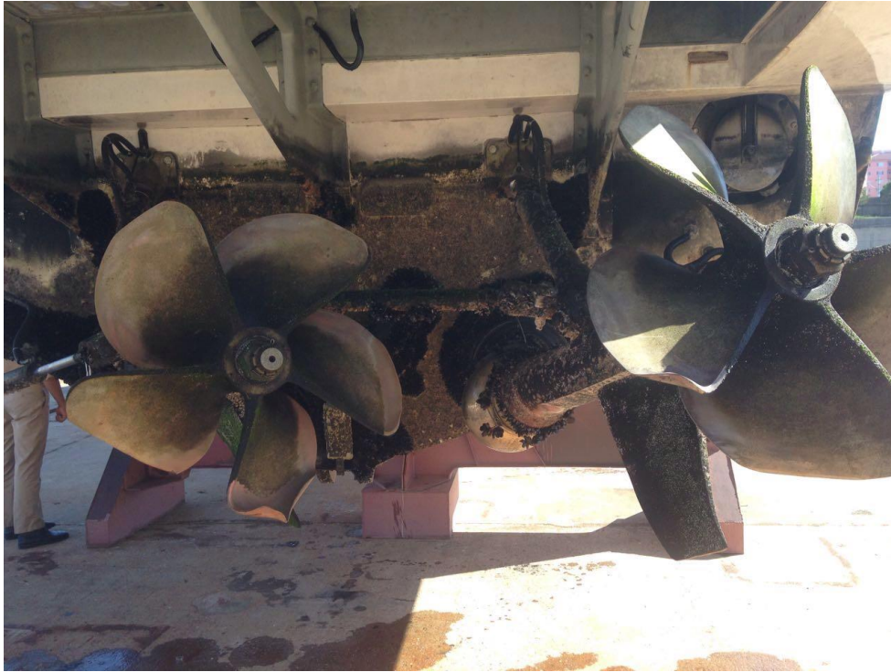
Picture 12: The damaged propellers of TCSG 25 Boat
