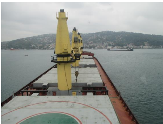
Pictures 22-23: Blind Sectors Formed By the Ship's Cranes
