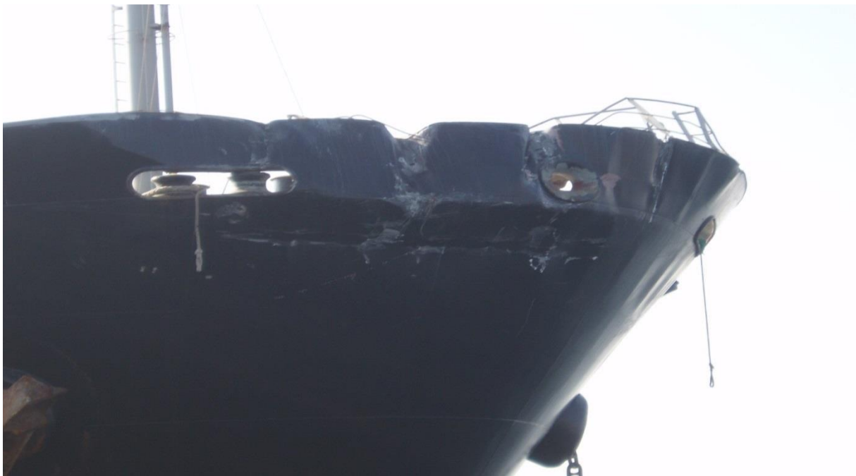
Figure 19: The Damage Occurred at the Bow of TANAIS DREAM
