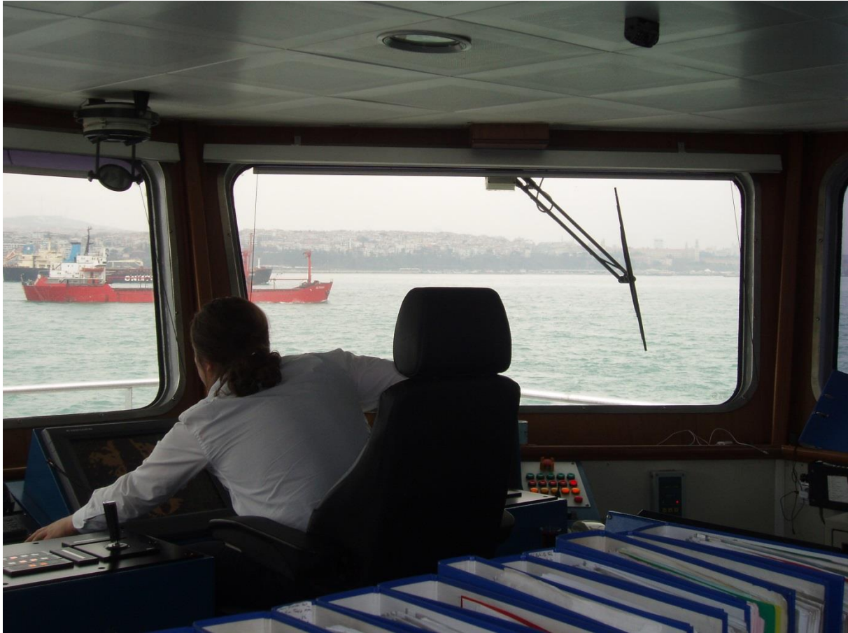
Figure 13: The Perpendicular Causing Blind Spot on the Bridge of SULTANAHMET
