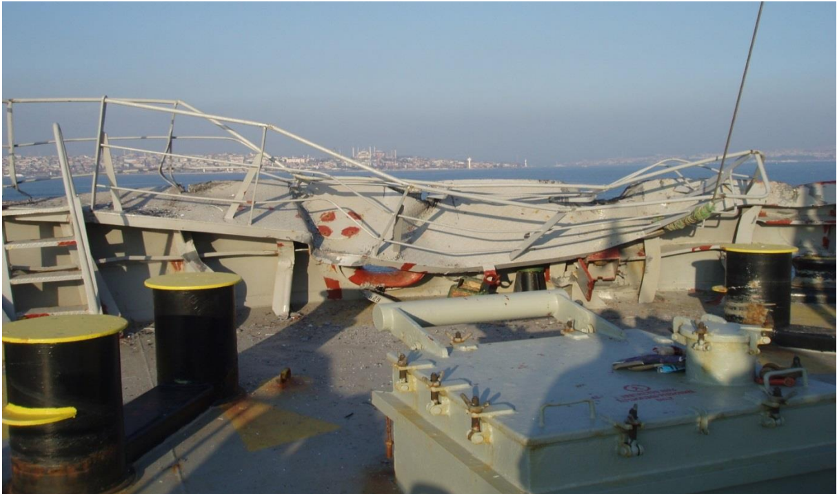
Figure 18: The Damage to the Forecastle of TANAIS DREAM
