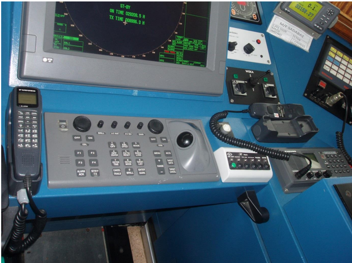
Picture 7 : Fixed VHF's on Bridge Control Console
