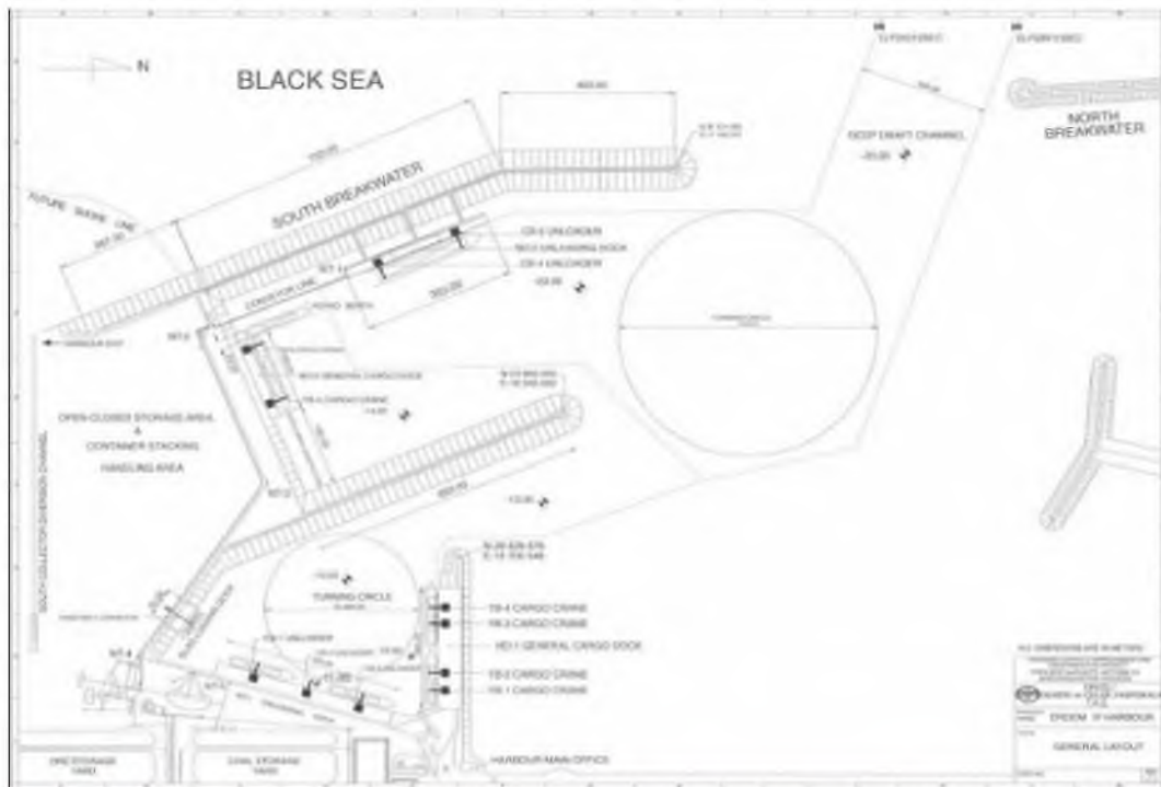
Figure 2 General Structure of Today's Port
