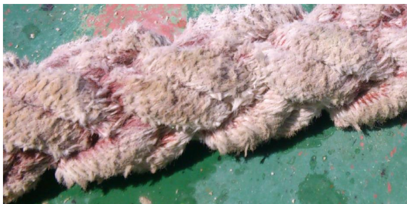
Picture 20: BODY of the broken ROPE
