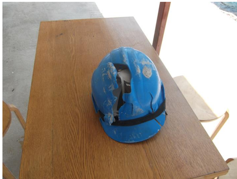
Picture 9: Helmet of the accident victim to whom the rope hit
