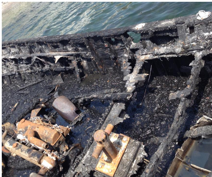
Figure 11: Damage caused to the Agent Boat SERDAR 2 after the Fire
