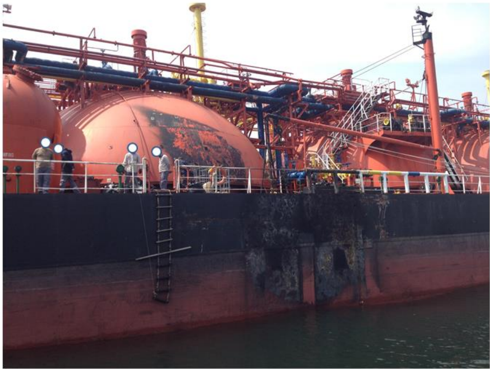
Figure 4: Fire Damage Caused to the vessel HABAŞ
