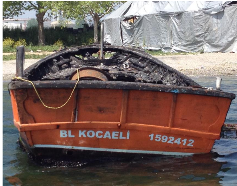
Figure 10: Damage caused to the Agent Boat SERDAR 2 after the Fire
