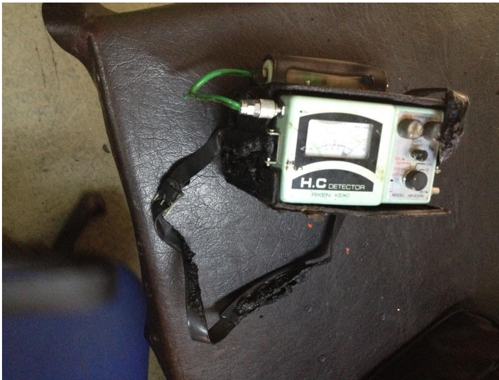
Figure 12: Gas Detector Damaged by the Fire
