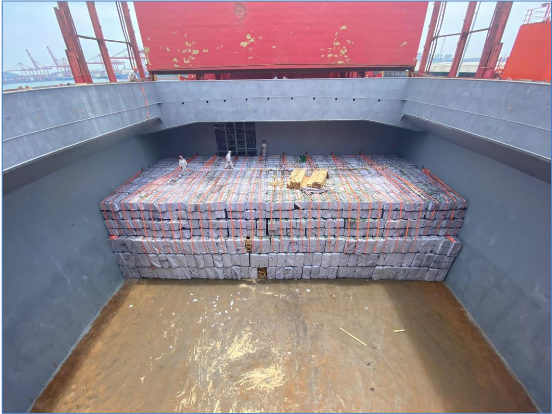
Image 7: A View from Hold Number 4 While Loading and Lashing Block Carbon Anode
