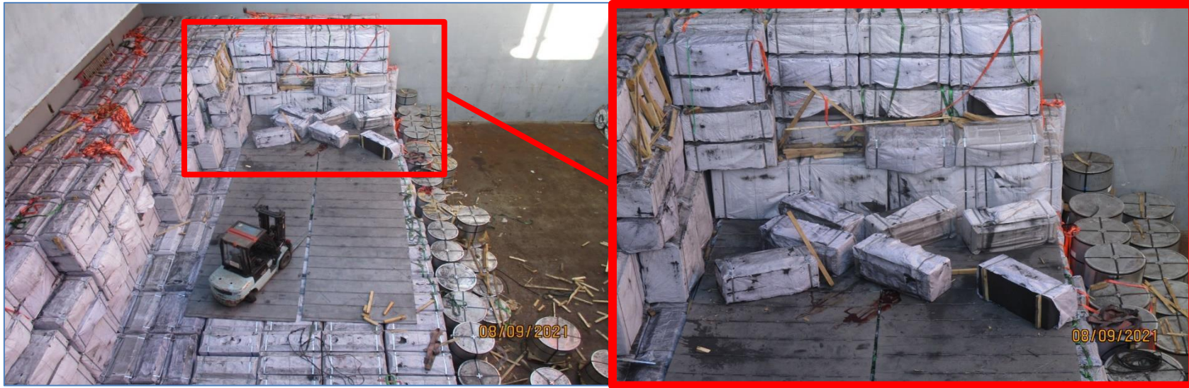
Image 10: Horizontal View of Fallen Cargo Block
