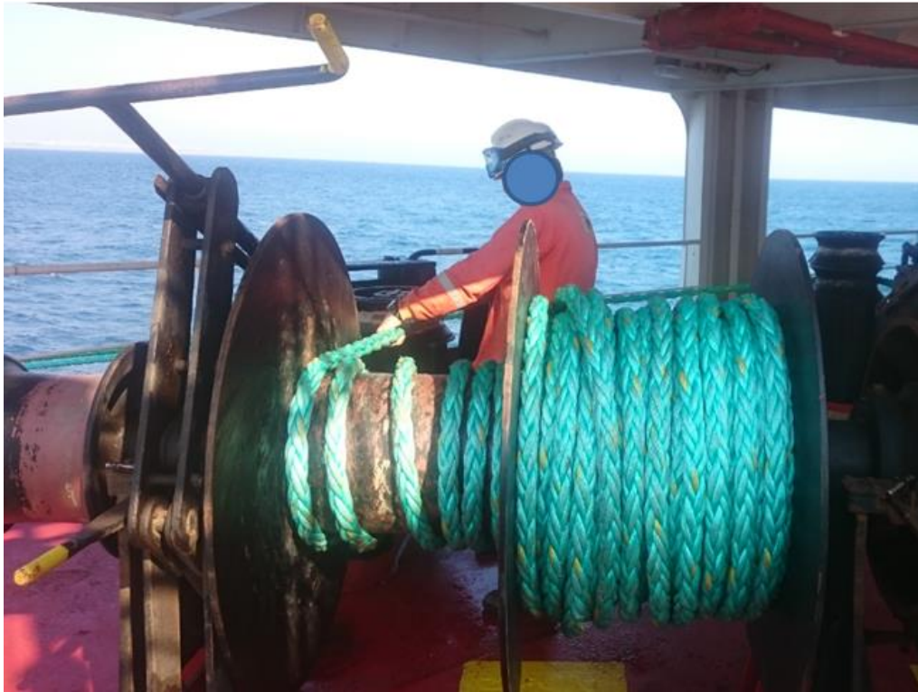
Picture 4: Pulling Mooring Ropes That Rubbed the Drum Disk by the Seamen
