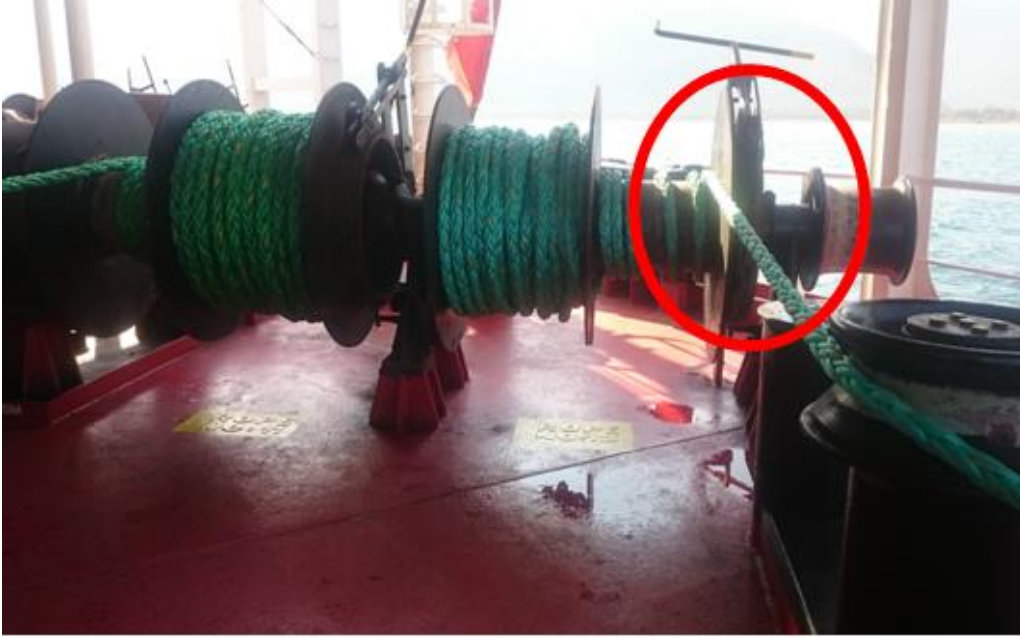
Picture 7: Rope Drum and the Pedestal roller fairlead Located on the Port Quarter of the Ship
