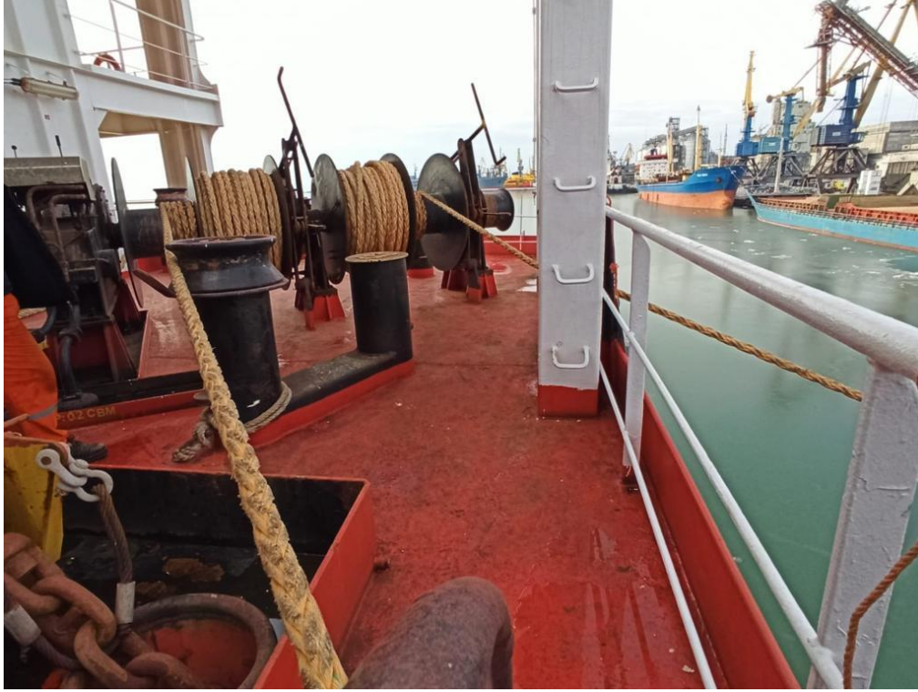
Picture 9: Hauling the Mooring Ropes Out According to the Mooring Plan
