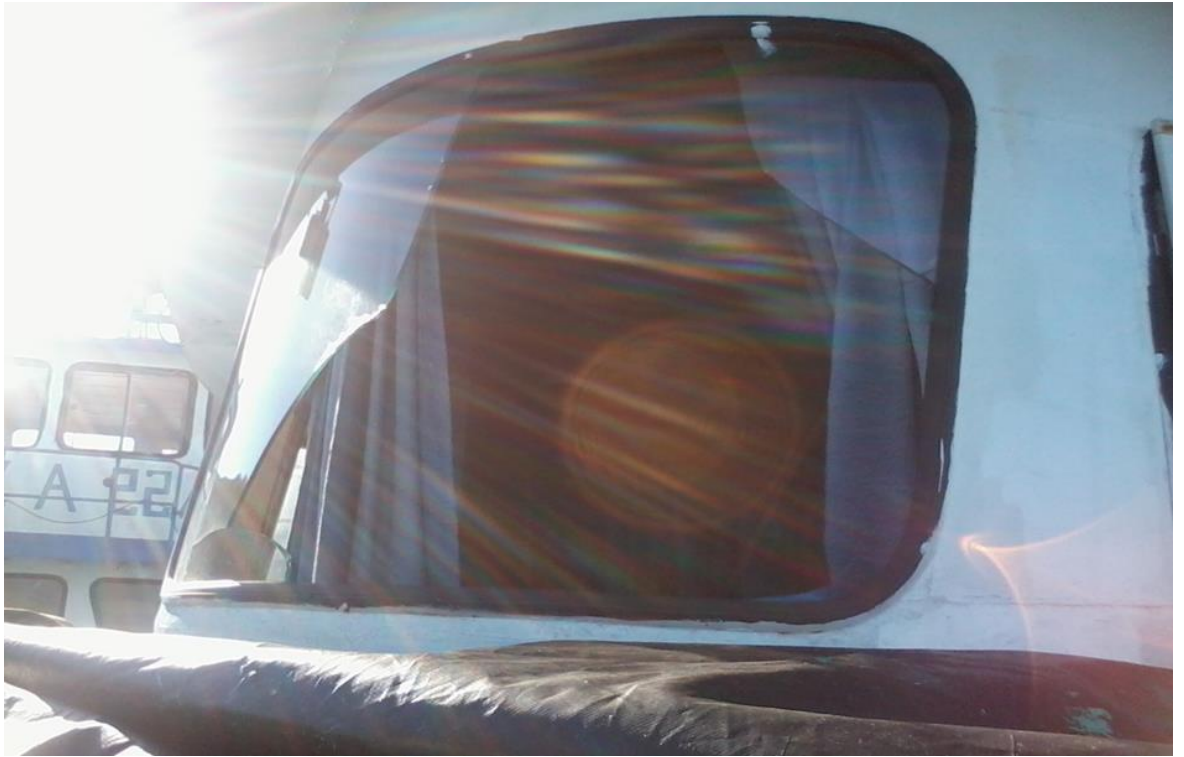
Figure 11: Damage on the Window of the Skipper's Cabin
