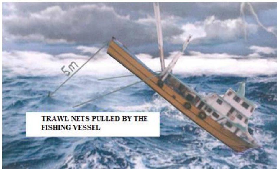
Figure 8: Representation of the Rising Aft of the Vessel With the Effect of Waves
