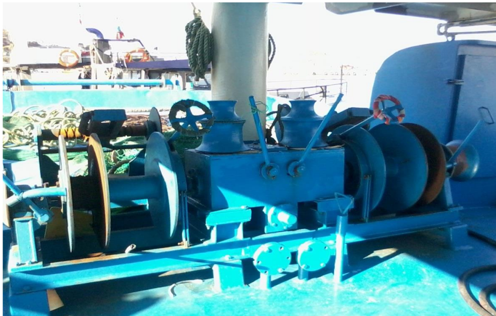
Figure 9: Windlass Used for Pulling the Nets
