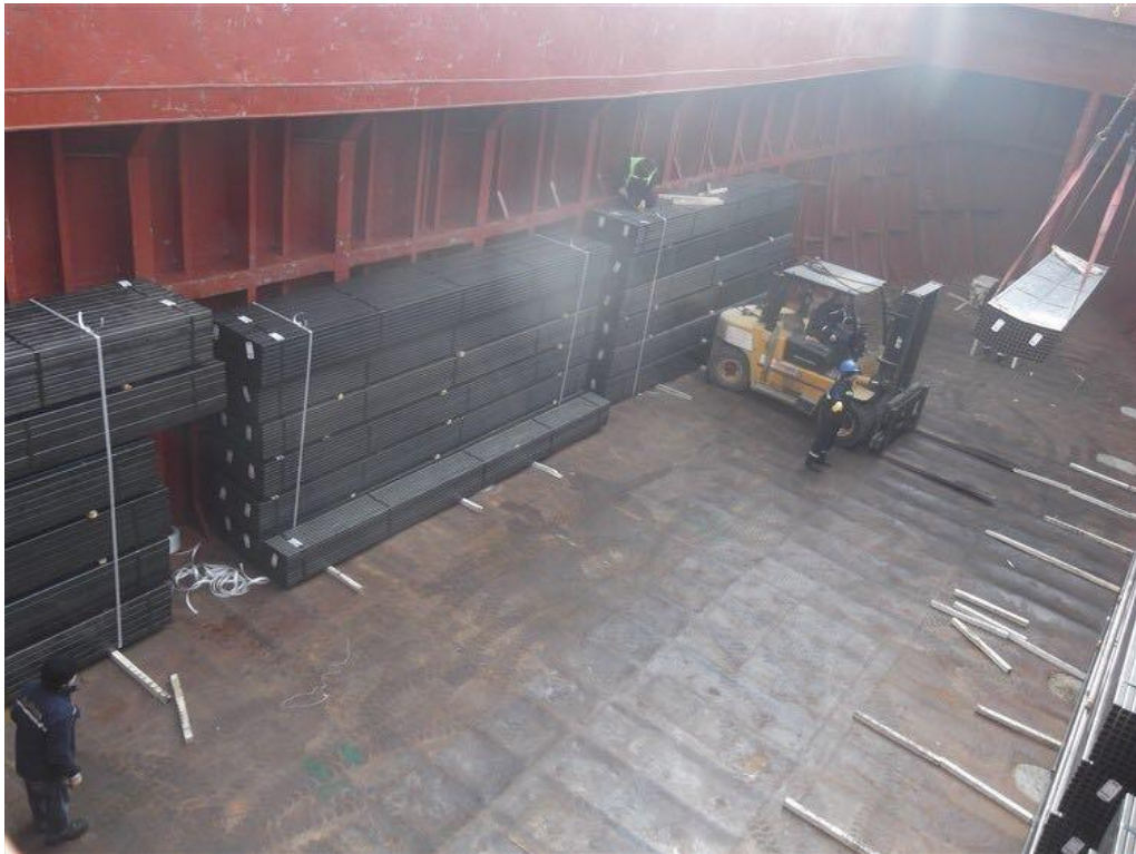
Figure 3: Lashing Continues While Loading on the Vessel ALİ OSMAN E.
