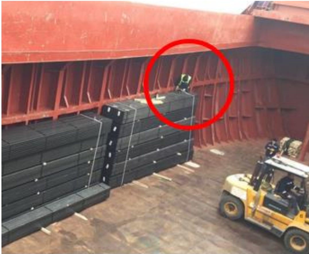
Figure 9: Lashing Personnel Engaged in Tying Down the Load to Itself
