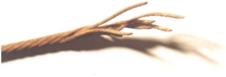
Figure 10: Typical View of the Parted Wire Rope Strand Caused By Corrosion Induced Wear 2
