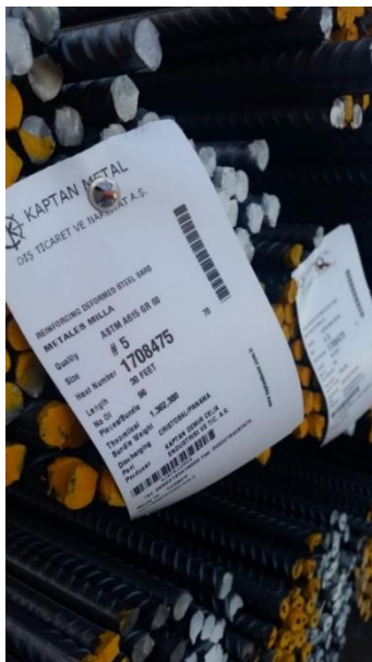
Figure 21: Label showing the properties and weight of one bundle of steel rebars
