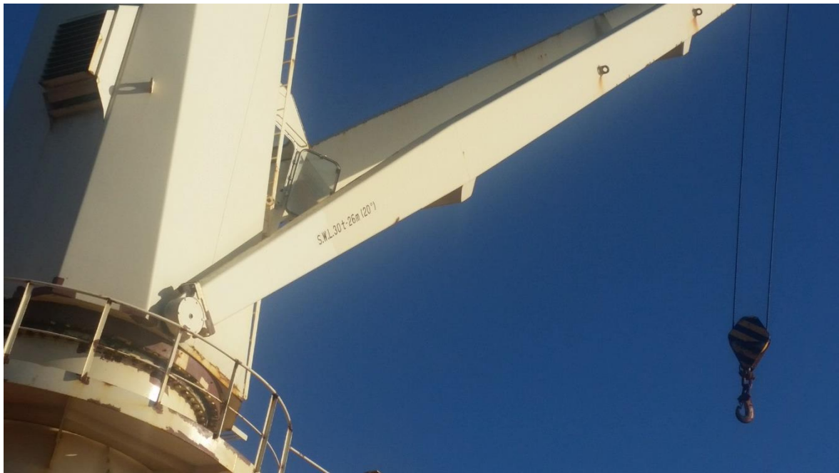
Figure 20: Safe Working Load and Radius of Deck Crane No.4 SWL 30t - 26m (20°)
