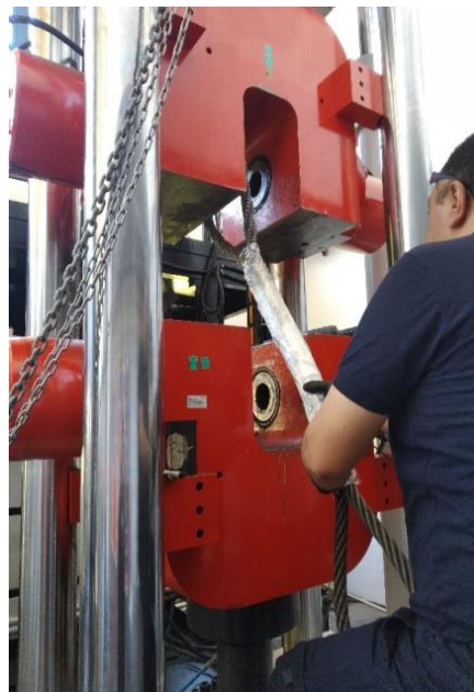
Figure 35: Preparation of the wire rope for the test
