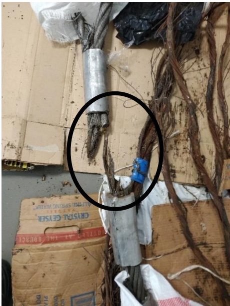
Figure 36: Section where the wire rope parted at the end of the test
