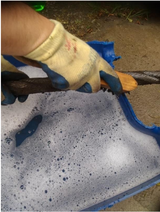
Figure 28: Cleaning of the lubricated wire rope with detergent
