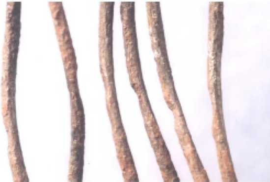
Figure 15: Wearing of the Metallic Part of the Wire by Corrosion Induced Wear
