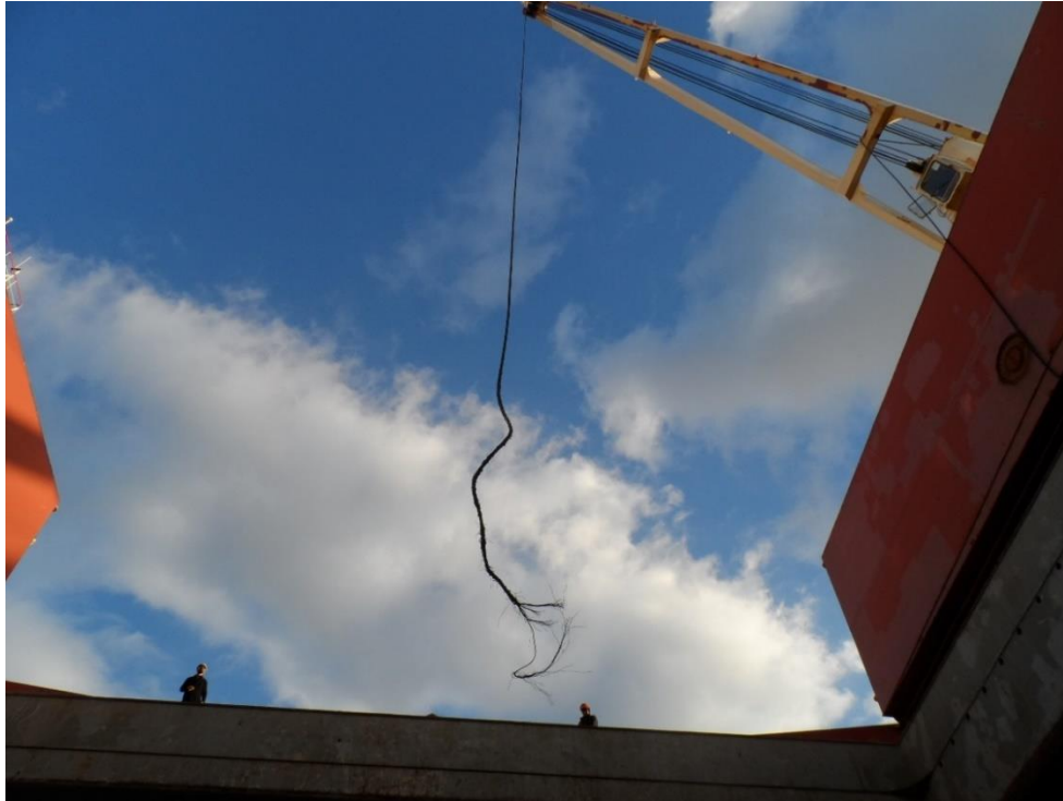
Figure 4: Photograph of the crane no. 4 and parted wire rope after the accident
