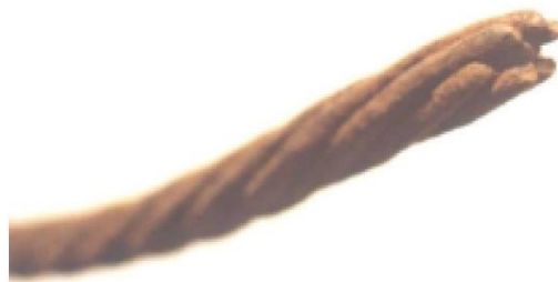
Figure 14: Typical View of Parting of a Wire Rope By Tensile Stress
