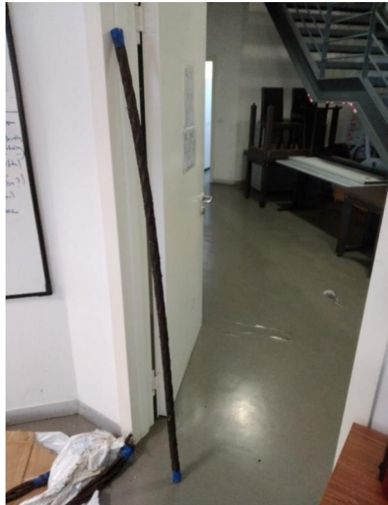
Figure 27: A sample piece of 184 cm. which is taken from the intact part of the parted wire rope
