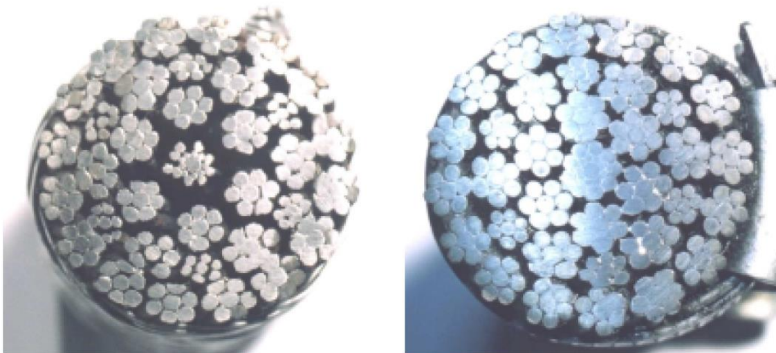
Figure 16: Cross sections of corroded (left) and "as new" (right) rope 6
