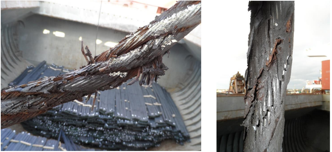
Figure 12,13: Photographs Showing Outer Lubrication and Inner Corrosion and Rusting of the Wire Rope
