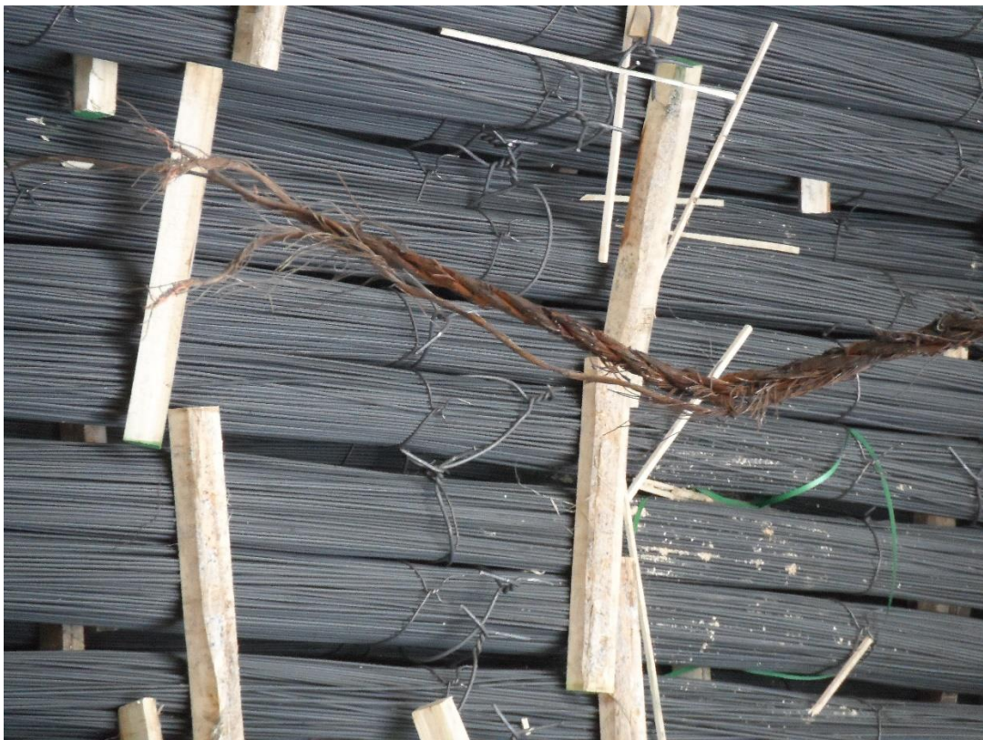
Figure 6: Photograph of the parted wire rope inside the cargo hold
