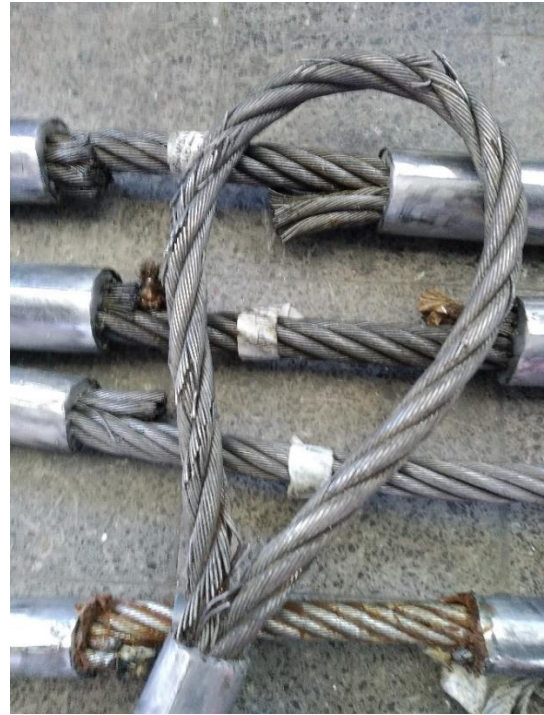
Figure 33: Photograph of the sent sample wire rope (breaks are apparent)
