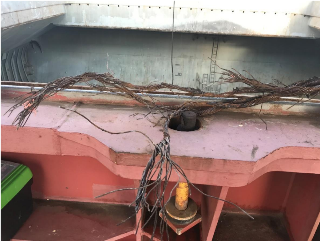
Figure 5: Photograph of the wire rope's strands and threads after the accident
