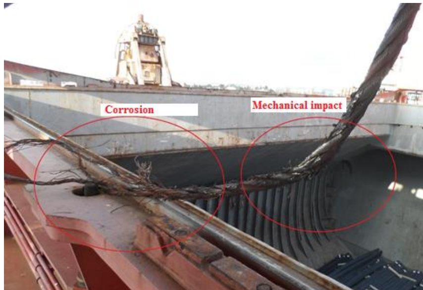
Figure 11: Parts of the Parted Wire Rope Exposed to Corrosion and Mechanical Impact
