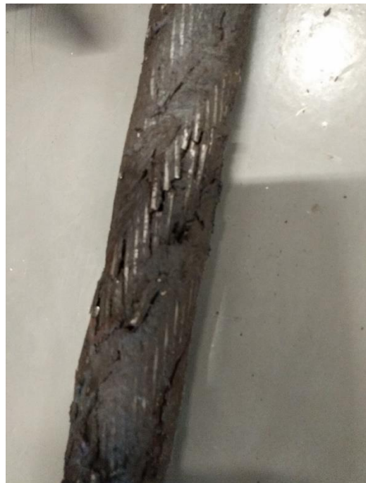
Figure 31: Breaks seen on the lubricated wire rope
