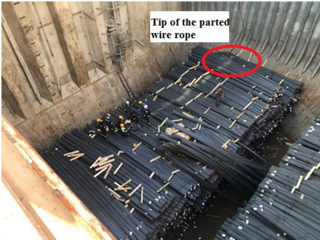
Figure 7: Photograph of the injured worker, parted wire rope and steel rebars inside the cargo hold
