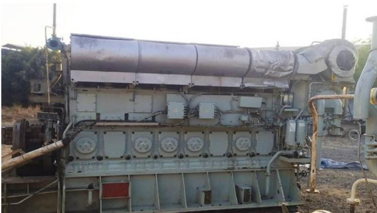
Image 9 Example for insulated twin main engine of FG SEVIL
